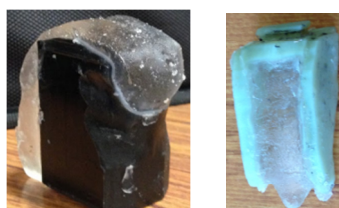
Figure 4. Compliant tongue (left) and soft palate (right) tissue inserts. These have a rigid frame on the exterior, which is part of the tissue anatomy.
