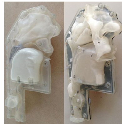
Figure 5. 3D printed airway model. Shown is one airway half with rigid inserts (left) and the completely assembled airway (right).
